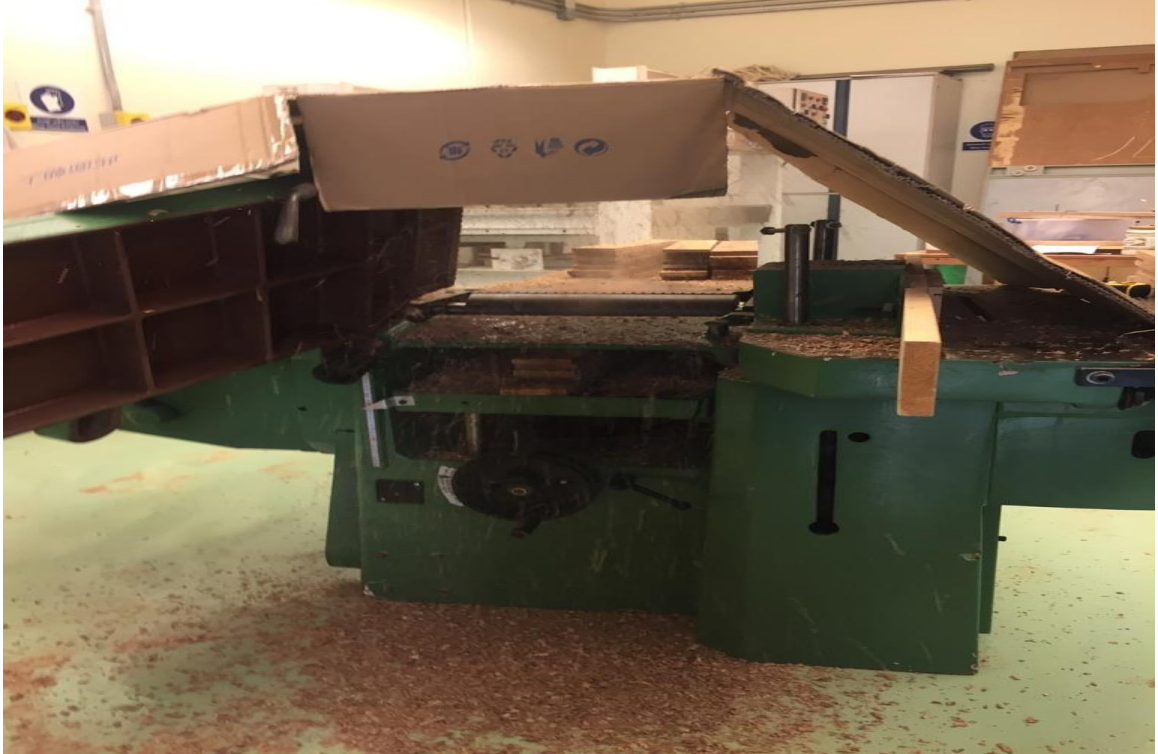
Figure 68: Cleaning and smoothing the surface of the wooden members
