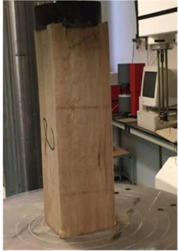
Figure 32 : Wedge split failure
