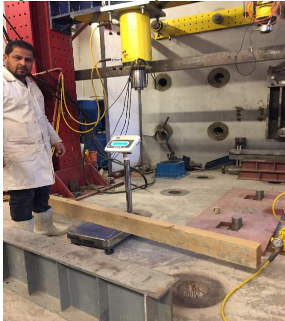
Figure 75: The wooden beam that was used to distribute the load over the truss.
