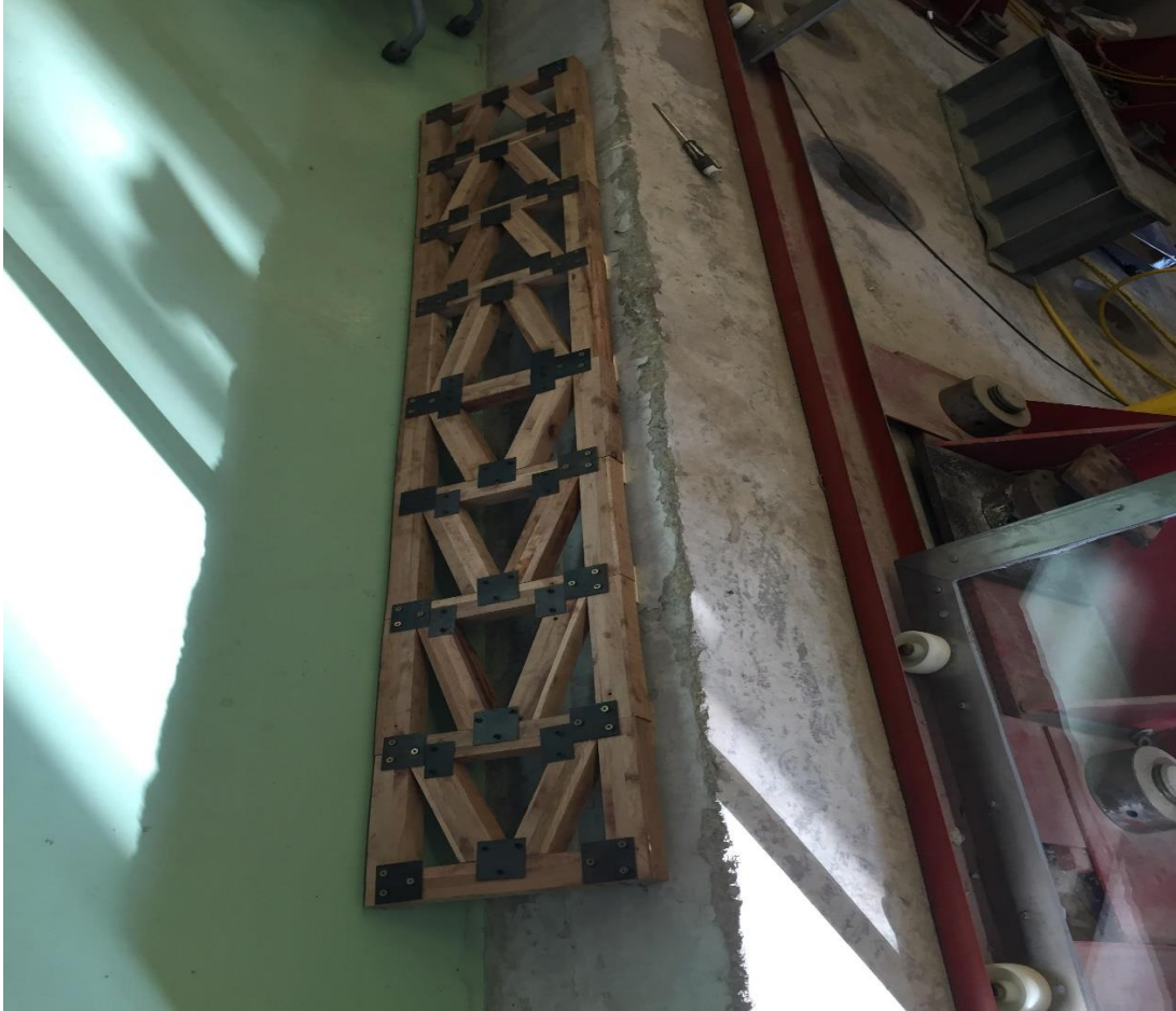
Figure 72: The truss final shape after connecting all the members
