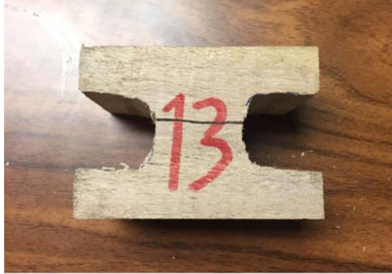
Figure 51: Tension perpendicular to the grain failure specimen
