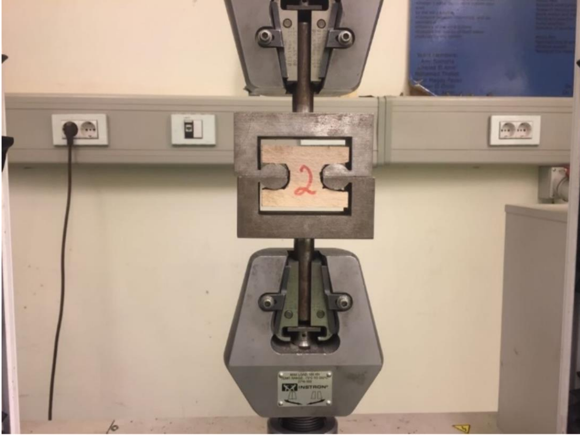
Figure 26: Tension Perpendicular to the grain test setup
