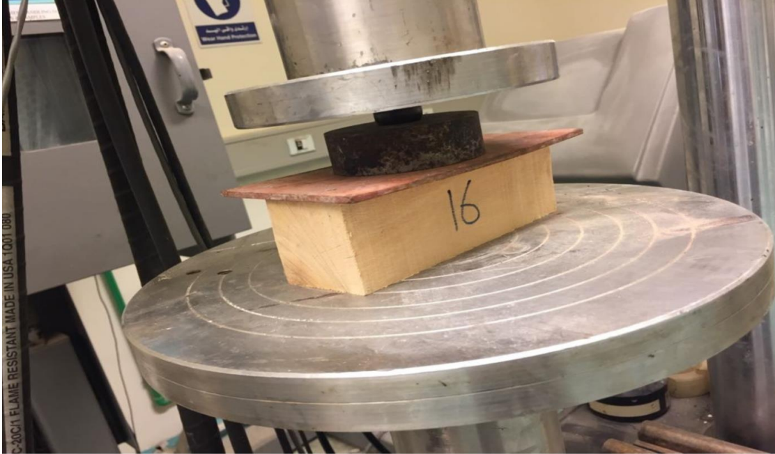
Figure 22: Compression Perpendicular to the grain test setup
