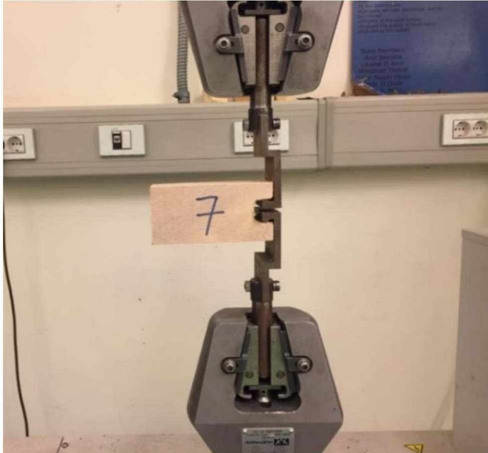
Figure 24: Cleavage test setup
