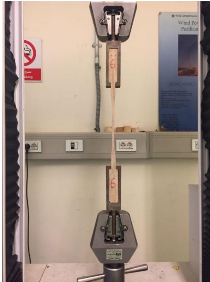
Figure 25: Tension Parallel to the grain test setup
