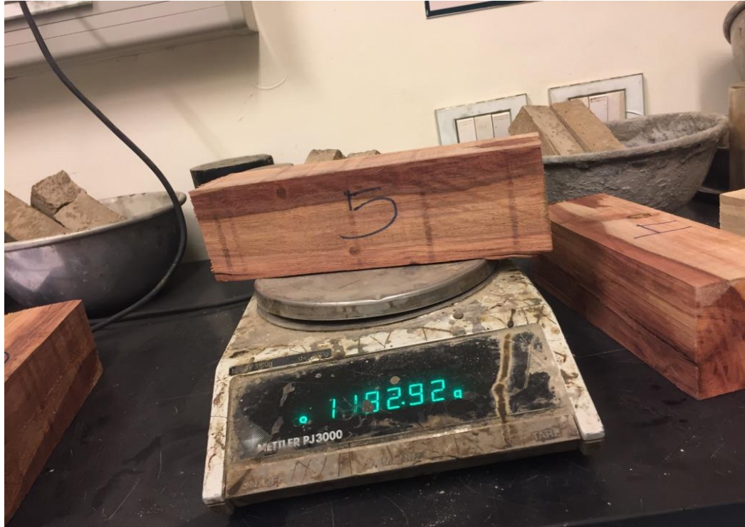
Figure 27: weighting the samples using a balance
