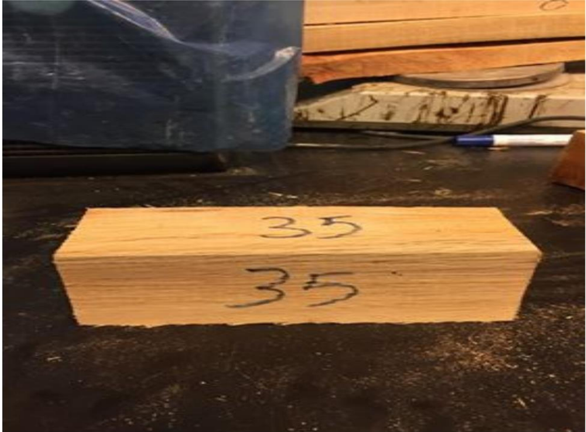
Figure 37: Compression perpendicular to the grain sample after testing
