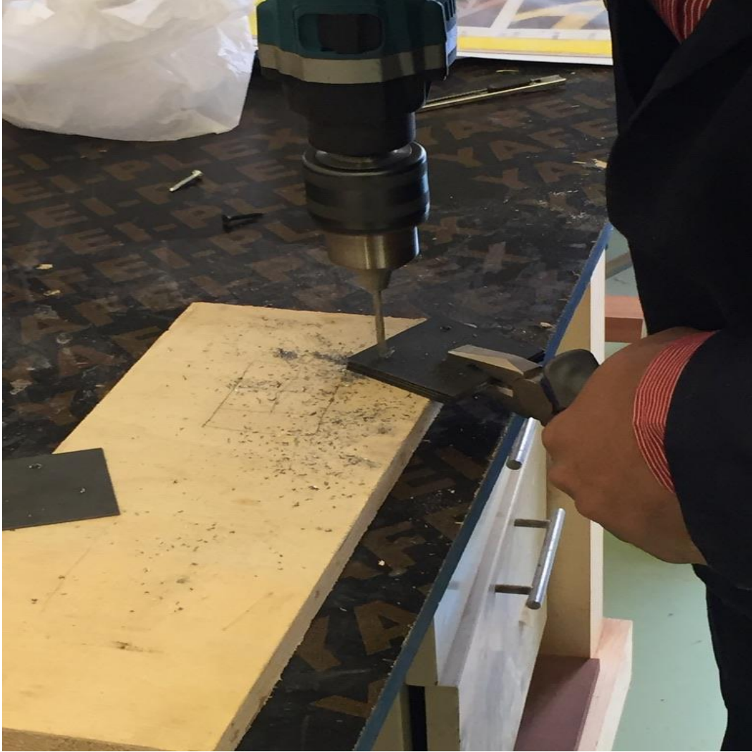
Figure 69: Making the opening of the screws using a driller
