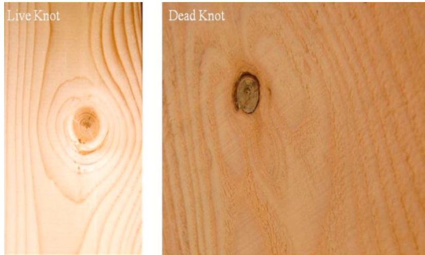
Figure 3: Dead and live knots in wood. (Kretschmann,2010)
