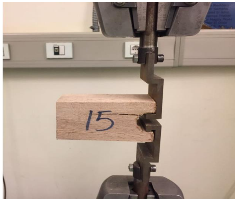
Figure 45: Cleavage sample after failure
