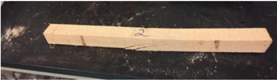
Figure 42: Cross grain tension failure
