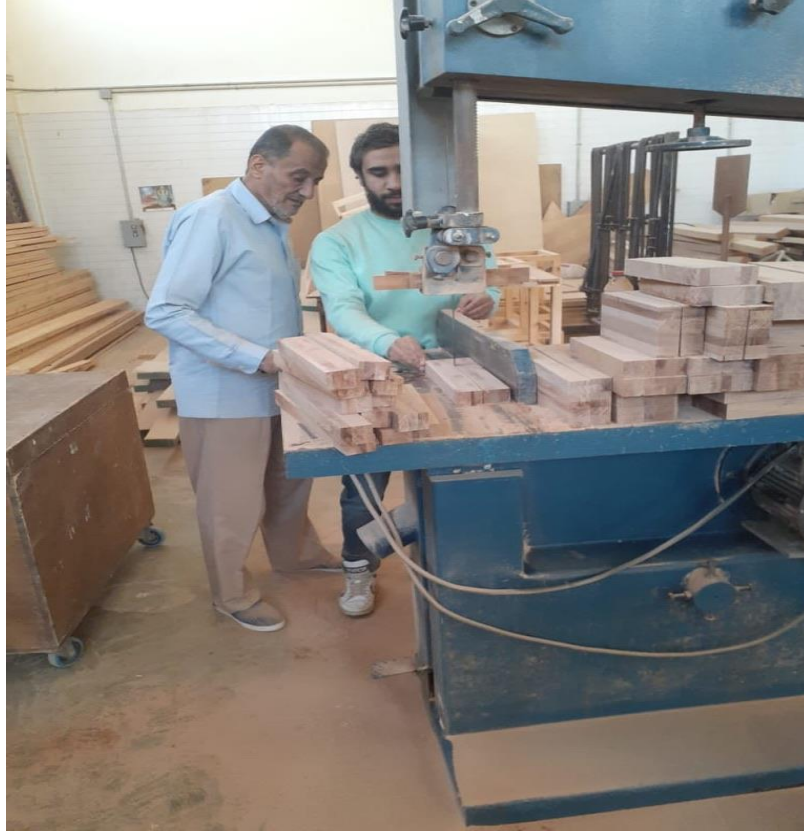
Figure 67: Cutting the wood samples into required sizes using electric saw
