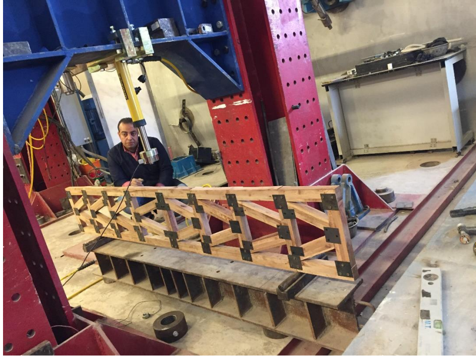
Figure 79: The supports used to support the truss
