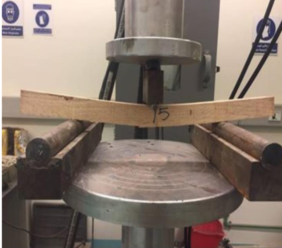
Figure 41: Simple tension failure
